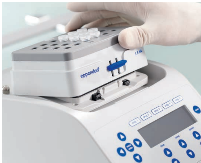
SmartBlock removal from Eppendorf ThermoMixer® C
