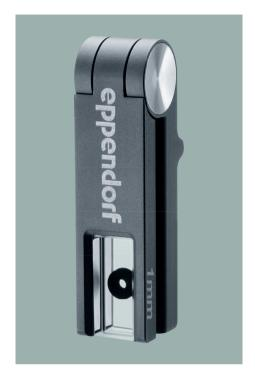
With an optical path length of only 1 mm, the  $\mu$ Cuvette G1.0 features a light path that is ten times shorter than the light path on standard cuvettes. This allows high nucleic acid and protein concentrations to be measured using the  $\mu$ Cuvette G1.0. Only 1.5  $\mu$ L of a sample is required for the measurement. The  $\mu$ Cuvette G1.0 offers a flexible expansion of the photometric application range of Eppendorf photometers.
