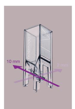
The patented\* Eppendorf UVette is a fully UV-transparent, single use cuvette made of clear plastic, with a light transmission of 220 nm to 1,600 nm. The unique design allows you to conduct flexible measurements with two different light paths (10 mm and 2 mm).
